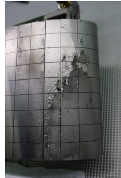
Erosion of JET Iter-like Wall
